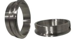
**V-Band Turbine Outlet Adapter:** The Garrett V-Band outlet adapter is for fabricating the turbo down pipe. This adapter mates perfectly with the G25 | G30 | G35 | GT30 | GT35 | GTX30 | GTX35 turbine housing outlet. It has a 3" recessed opening feeding the flange.
