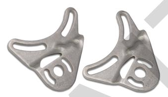
**Adjustable Wastegate Bracket:** The Garrett Adjustable Wastegate Bracket allows for a greater range of motion to set up the compressor outlet and wastegate can. The bracket also allows for redirection of the actuator to keep vacuum lines away from heat or sharp edges. The adjustable actuator bracket is available for use on GT25R, GT28R and GT30R turbochargers.
